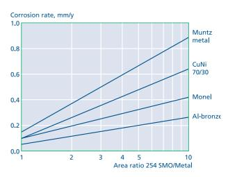
*Fig. 11.* Galvanic corrosion of copper alloys in slow moving seawater at ambient temperature.
