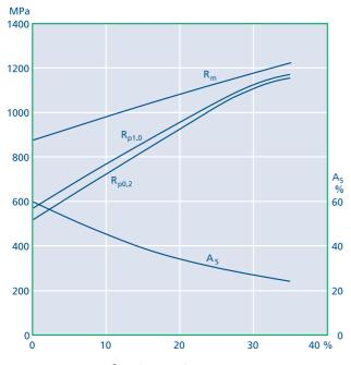
*Fig. 13.* 654 SMO<sup>®</sup> – influence of work hardening on strength properties.
