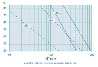
*Fig. 8.* Risk of pitting and crevice corrosion on conventional stainless steel in water of different chloride content or temperature.
