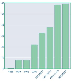
Fig. 7. Critical crevice corrosion temperatures (°C) for some stainless steels in 6% FeCl<sub>3</sub>. Testing according to MTI-2.
