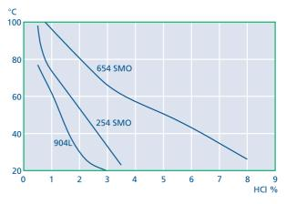
Fig. 3. Isocorrosion curves, 0.1 mm/y, in pure hydrochloric acid.
