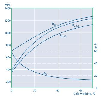
*Fig. 12.* 254 SMO<sup>®</sup> – influence of work hardening on strength properties.
